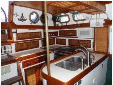
Galley - The galley has forward-facing double sinks with hot/cold pressure water, fresh water foot pump, and saltwater foot pump. The stove is a three-burner Seaward Princess LPG with an oven. There are two refrigerators. Under the companionway is the Frigoboat keel cooled box which is lined with vacuum panels. It has both top and side access doors. A secondary refrigerator – Grunert Polar Mate – in the aft corner is
