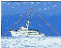
ground plate at least 1 square foot in dimension. It is important that you ensure that your crew fall within the protection of the "cage," something not always feasible when the vessel is not built of steel or aluminum. On fiberglass or wooden boats it is advantageous to have a mast or other conductive metal protrusion extending well above the vessel, creating what is known as a "cone" or zone of protection.
