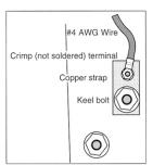
A metal keel makes an excellent ground for a lightning protection system. Bottom paint does not act as a significant barrier to a strike that has gotten this far in its quest to reach the water.
