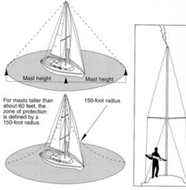
As long as the boat is entirely within the cone, there is little risk of anyone aboard being struck directly. However, you are still at risk if you are touching metal, and especially if you are bridging two metal components—the wheel and a stanchion, for example. And if the mast is poorly grounded, side flashes—a leap from the mast to other parts of the boat—can also cause injury. Even with a good ground, it is wise to stay well away from the mast during an electrical storm.
