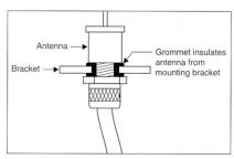
Often you will find that the connection is through the mast, usually due to contact between a masthead antenna bracket and the coax shield. You can break this connection by installing insulating grommets around the bracket mounting bolts or in the antenna-mount hole.
