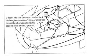
Isolate bonded tanks by inserting a section of rubber hose in the fuel line. The propeller and shaft are easily isolated with a flexible coupling. (Note: A zinc collar is still required to protect the bronze prop if the shaft is steel.)
