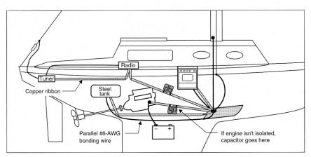
If other metal components bonded for lightning protection are also connected to the RF ground system, disconnect RF connections from the components to the radio and make them to the ground plate. Configured this way, a single capacitor will separate the DC ground from the RF ground. If your foil is thick enough—at least 9 mils (0.009 inches)—you can substitute the ribbon for the wire; otherwise connect the ribbon parallel to the #6 AWG bonding wire.
