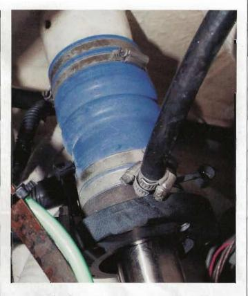
Lip-type stuffing boxes such as the one shown here offer long life and reliable operation, provided they are properly installed and maintained. The manufacturer's installation instructions must be followed to the letter, particularly the specifications concerning the water injection hose and its fittings.
