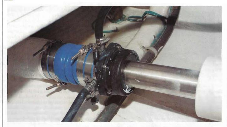
A lip-type seal installed in a twin-screw vessel. This installation includes a spare seal carrier that is located directly forward of the stuffing box. To avoid damage, there should be more separation between these two components; the spare seal carrier spins with the shaft, while the forward end of the stuffing box does not. The dual water injection hoses ensure adequate lubrication in the event that one engine fails and causes one shaft to "windmill" (or spin) while the engine is not running.
