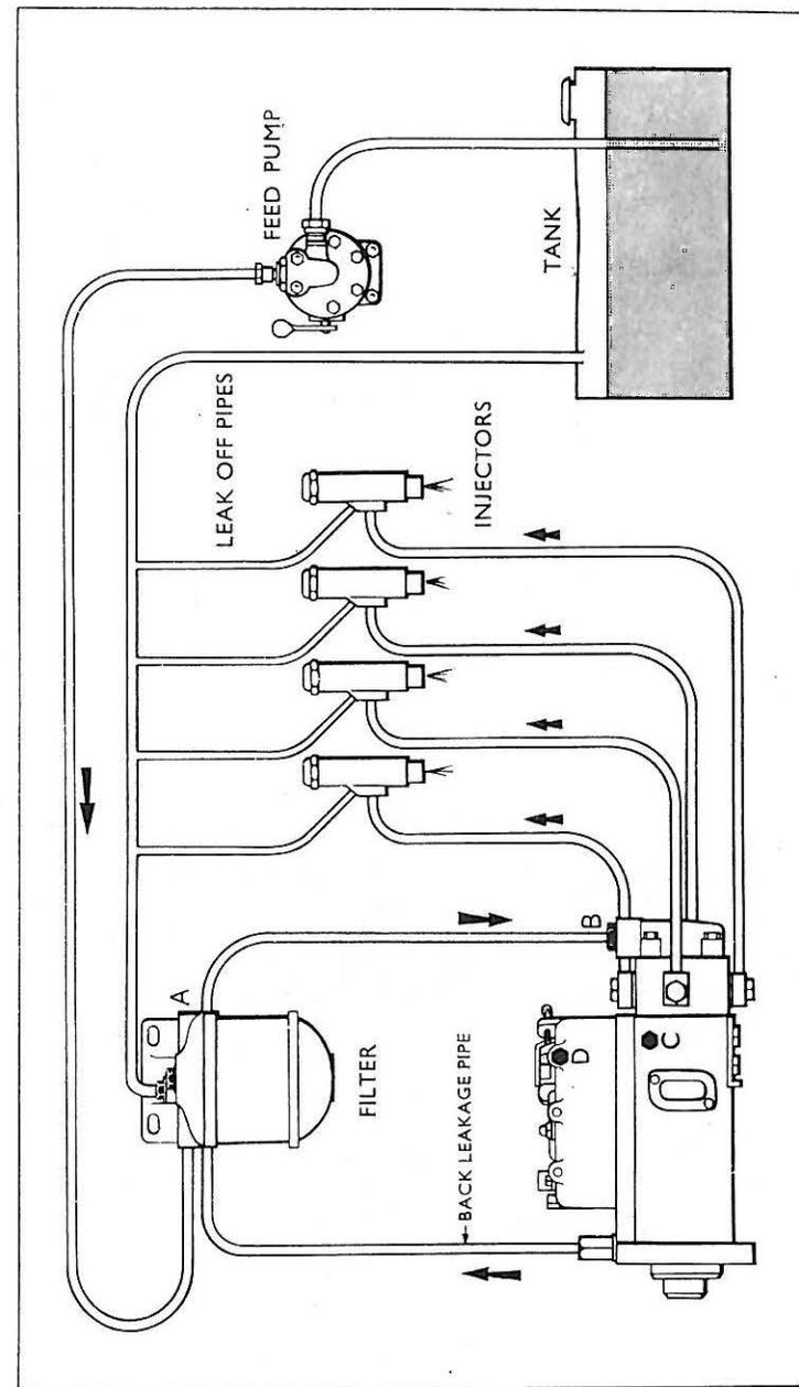
Fig. 4. Typical fuel system with lift pump
