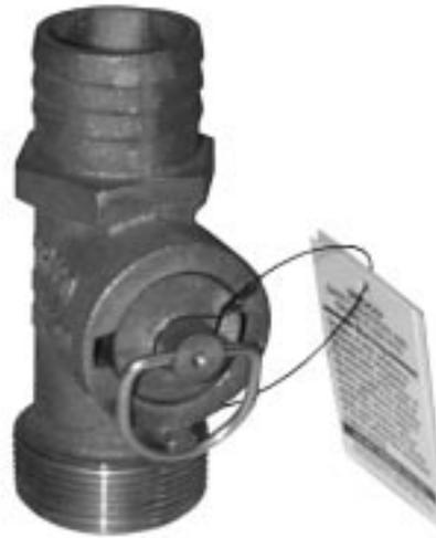
**Maintenance:** Remove the Quick Release Plug monthly and lubricate the O-Rings with TFE or Silcon Based grease. Do not use petroleum based lubricant.
