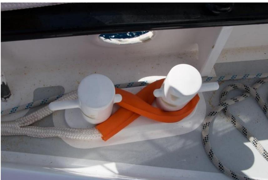
**Novara's** aluminium hull has substantial bollards. Note the chafe protection and figure of 8 loop to stop the bridle jumping the bollards when the load comes off the bridle.
