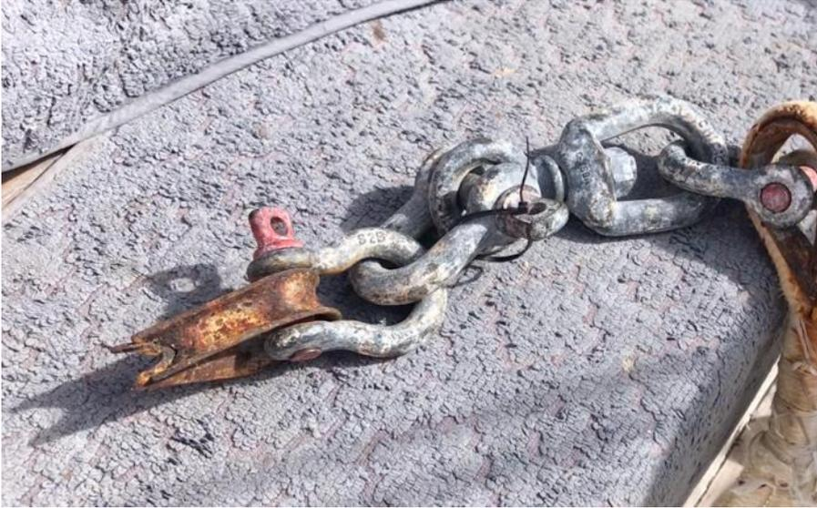
*“A few hours later, I was still below and clearing away the carnage when I felt Mo’s motion had changed. Suddenly we were lying ahull. I dashed on deck to find that only the bridle part of the JSD was still attached to the boat; the drogue had parted at the lead eye splice.” RR*
