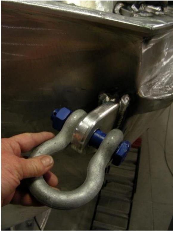
**Susanne Huber-Curphey** has 20mm thick and 90cm long aluminium plates welded to the hull to be used specifically as anchor points for her JSD.
