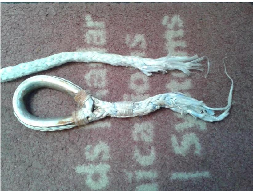
UV degradation is concern so wherever possible the exposed sections of the bridle leg should be protected whenever the bridle is exposed to the sun.
