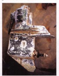
If you want to see what would happen to an anodic fitting if it wasn't protected, look at a wasted anode. In this case, the anode (zinc) is long gone, so that the aluminum outdrive, or what's left of it, looks like a wasted anode. Note that corrosion is not covered by insurance.
