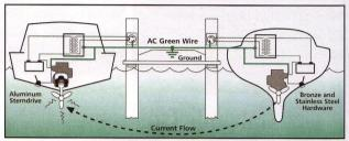
When two or more boats are connected to shore power, one side of the necessary circuit required to form a galvanic couple is provided by the AC green grounding wire, which is also connected to the boat ground system, engine, and underwater hardware. The seawater electrolyte provides the other side of the circuit. Galvanic current flowing around the circuit will corrode the least noble metal between the two (or more) boats, in this case an aluminum sterndrive.
