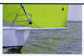
[TACKLINE] In light winds, fully trim the tackline to set the tack snug on the end of the bowsprit. This shortens the luff, which is optimum for sailing tighter reaching angles.
