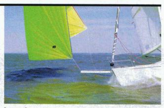
[TWING] On most boats, a twing (block-and-tackle led to the rail) is needed to control the height of the spinnaker sheet. But on the 105, the boom acts as a natural twing.
