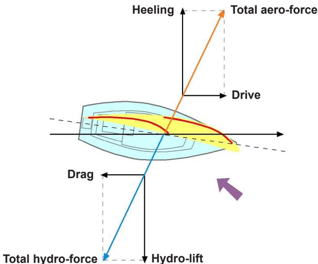
The relationship between these forces determines 'helm balance' – whether good or bad. Now look at the illustration on the right – the same boat side-on, with the centres of drive and resistance marked on the sails and hull respectively. It's easy to see how the boat will heel but, since the two forces are vertically aligned, there's no tendency to turn, either to windward or leeward. The boat is said to be perfectly 'balanced', offering a very easy life for both human and mechanical helms.
