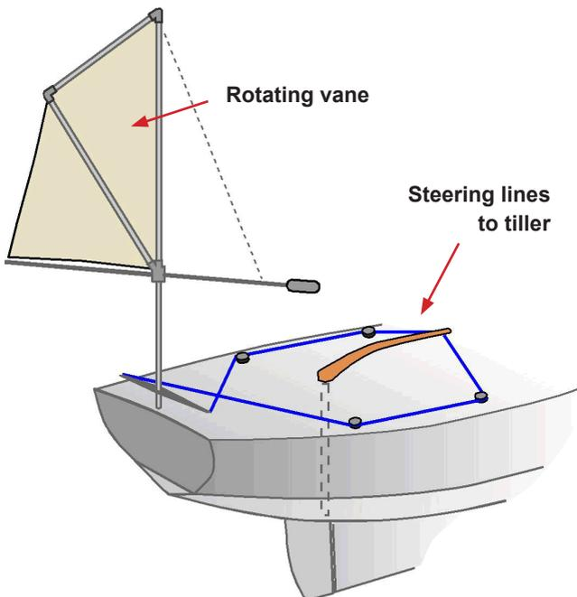
***Meet Miranda – whose primitive approach to self steering must have been sorely taxed overcoming the friction in Gipsy Moth's primary steering system***
