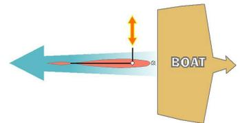
**2** *The boat strays off course. The vane senses the change in direction and turns the tab in response*
