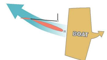
**NOTE:** Although not usually obvious, all modern vane gears use some form of feedback mechanism to tame excessive responses to course changes. Otherwise called 'yaw dampening' – a phrase that explains the objective perfectly.
