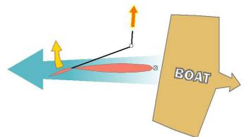
**3** *Driven by the tab, the rudder swings over. Because the link from the vane linkage is aft of the rudder axis, the tab straightens progressively. With the boat now returning to its course, the tab's effect is now zero and the rudder will turn no further under its influence.*
