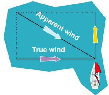
In the next illustration, the skipper decides he would like to sail closer to the wind so alters course until the true wind is  $45^\circ$  on the bow. Remember that nothing has changed except the course. For the vane, on the other hand, quite a bit has changed. The wind has strengthened to over 15 knots and is now only a little more than  $25^\circ$  off the bow.
