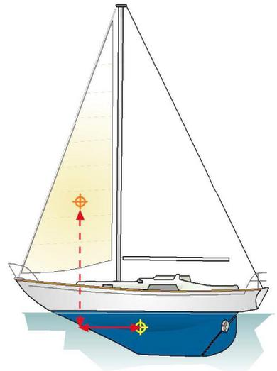
*On well-designed boats with sails in at least fair condition, minor tweaking of the sails will neutralise the helm. Weather helm can often be reduced by easing the mainsheet, while easing or taking a roll in the mainsail will help reduce lee helm. So...*
