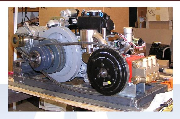
After determining where everything would be mounted, it was disassembled for painting. I use POR-15 which was touted as an engine paint that was tough and heat resistant. It also was suppose to treat the metal and prevent rust. We shall see.
