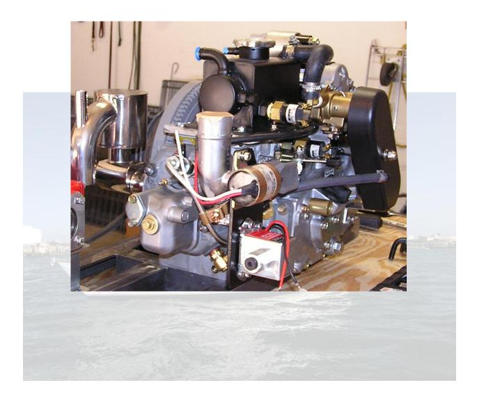
I built a base to mount the engine, pump and alternator on and then laid out the positions. It is a simple angle iron frame. The engine and high pressure pump are bolted directly to this frame. The alternator is mounted on a mount welded to this frame, the mount and adjustment arm was supplied by Zena the manufacturer of the alternator.
