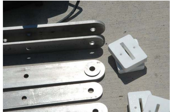
Raw plates after cutting Note Starboard™ blocks which will become the covers
