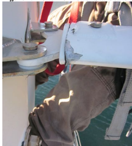
Figure 2. Trailing edge damage. Lower Stbd Spreader
