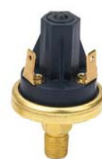
LF20-121210-1 Pressure Switch 0.25 PSI N.C. (will open with ~ 9" head of diesel)
