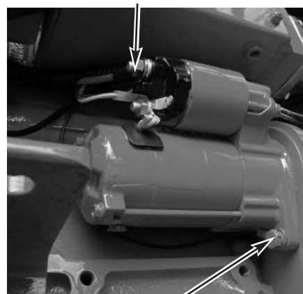
Typical start battery negative
