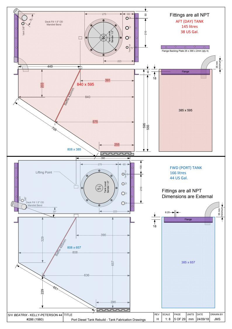
The flanges at the top of each tank rest on the bearer beams. Studs are welded at the top of the tank to fasten the flange to the tank. Flange mounting holes are ovals to allow for vertical adjustment. Once the tank is in place the flanges are bolted or lag-screwed to the bearer beams and then bolted to the studs.
