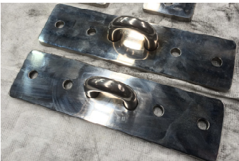
Preventer line passes through custom-built 12mm padeye.
