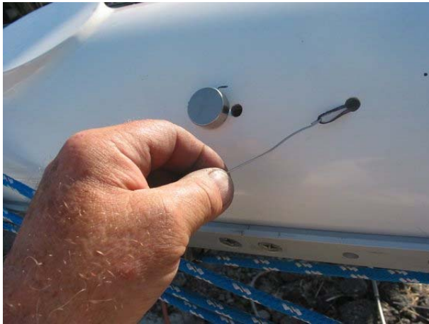
Figure 6. A wire hook is used to snag the twine which has been dragged past the holes by the magnet (on the outside) and the steel nut (on the inside) to which it is tied. The far twine will be hooked next. The colors tell you which line goes to which hole.
