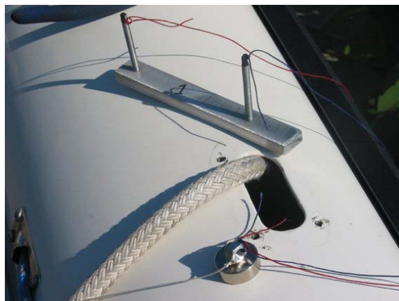
Figure 4. The backing plate ready for installation. The steel nut atop the cylindrical magnet will drag the lines along the inside of the mast, following the magnet which is on the outside.
