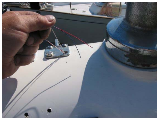
Figure 4. Pulling the backing plate into place.
