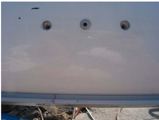
Figure 10. With temporary holding screws in place, a hole was drilled for a pop rivet which now fastens the backing plate in place. An alternate method is to drill and tap for a small machine screw.
