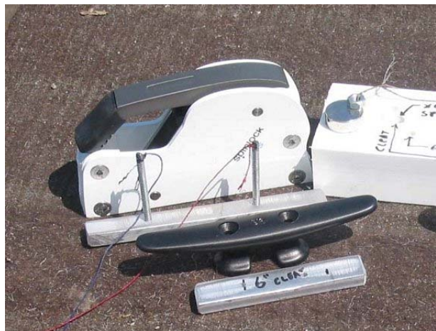
Figure 1. A cleat and a line clutch with their backing plates ready for installation. The white block of 2" Starboard™ was used as a drilling alignment block.
