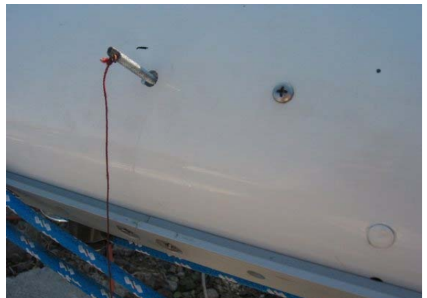
Figure 9. While holding tight to one alignment rod, the other is removed and a temporary machine screw is used to hold the backing plate in place. Remove the final alignment rod and add a temporary screw in the second hole.
