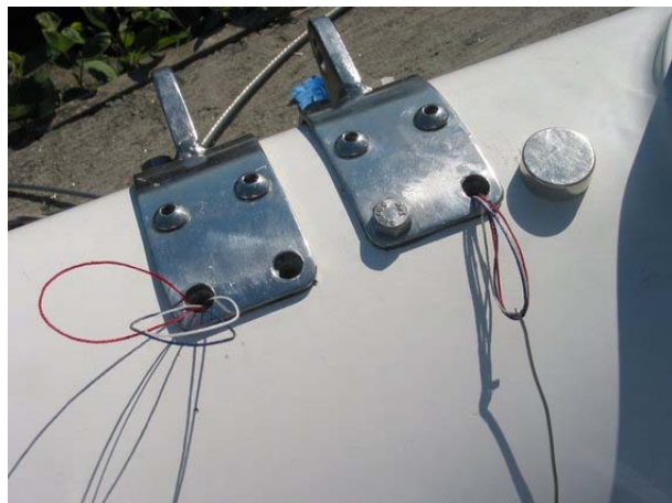
Figure 2. The twine is extracted with a wire hook once the magnet/nut combination is moved past the mounting holes.
