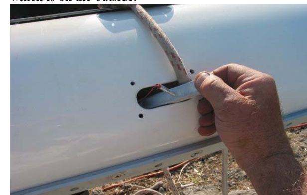
Figure 5 (alternate). Inserting the backing plate into a halyard exit opening. Note the red and green seizing twine attached to the threaded alignment rods.
