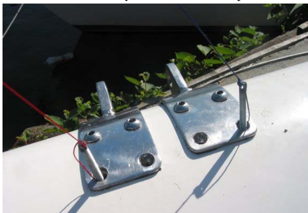
Figure 5. The alignment rods in place, still screwed into the backing plate.
