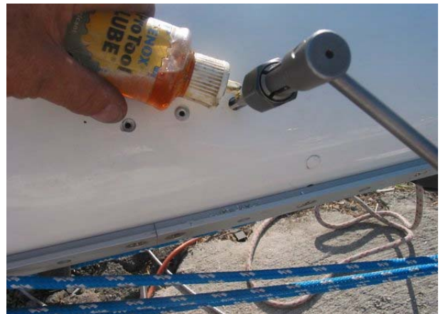
Figure 11. Tap and drill to the proper size for the permanent mounting bolts. Use tapping fluid and a new tap.
