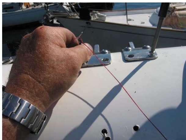
Figure 6. While holding one rod tight, remove the other and screw a temporary fastener in place.
