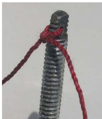
Figure 3. Close-up of the end of the alignment rod showing the flange and hole drilled for the twine.
