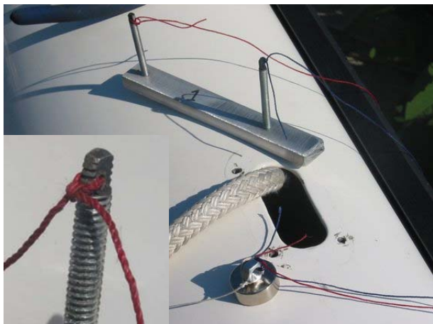
Figure 1. Backing plate components ready for installation. Note round heavy duty magnet, colored twine, and "alignment rods" with flanges. The steel nut atop the magnet will drag the lines along the inside of the mast, following the magnet on the outside of the mast.
