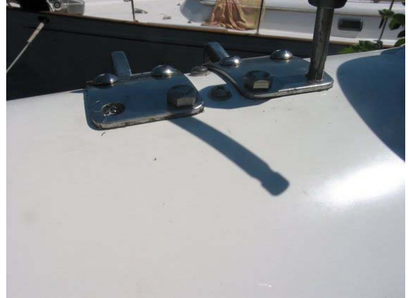
Figure 8. With the temporary fastener removed and the outer holes are drilled and tapped. This step is repeated for the other outer hole (to left) and the job is complete.
