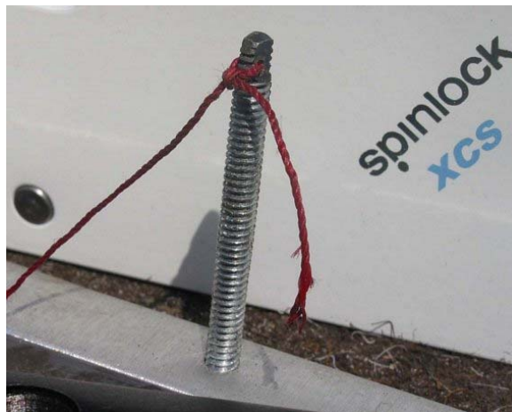
Figure 2. One of two "alignment rods" is inserted in the backing plate.
