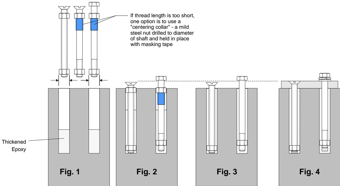
Fig. 1. Drill oversize holes using the hardware to be mounted or a template. Always "dry fit" the hardware, then wax up the nut and the bolt. Partially fill the hole with thickened epoxy . It is a good idea to wet out the hole first with unthickened epoxy.
