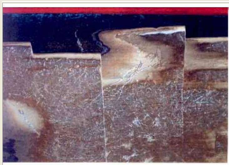
Fairing material that either turned soft or was not properly mixed and catalized. Scrape marks were made with the end of a ball point pen to indicate how soft is is, a perfect environment for blister formation. This is the pointit where the bottom was faired into the old gelcoat at the boot stripe. Note blister voids at lower center.
