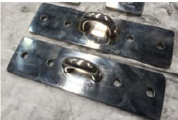
Preventer line passes through custom-built 12mm padeye.
